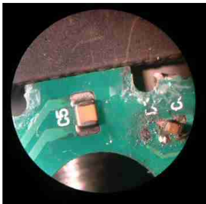
C5 is to be replaced.
