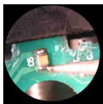
A small soldering iron tip has been chosen to work with this capacitor. Solder is added to the capacitor contacts.
