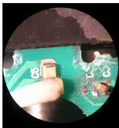
A cotton bud is used to wipe IPA and rework flux over the solder contacts.
